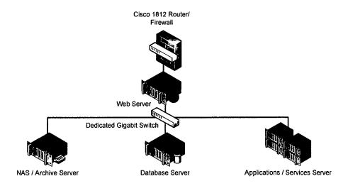
With the web server managing the end user interfaces, the database server managing the data, the applications server managing the communication between the file systems and message queues, and the archive server managing the redundant backups, the system functions smoothly and efficiently for the current user base.
