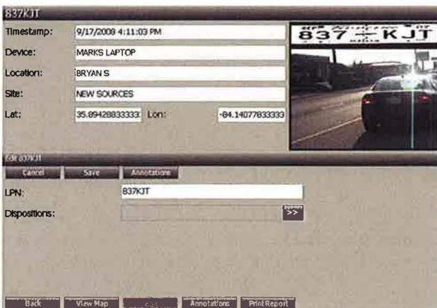
Use the "Edit" button to correct the plate text and/or assign a disposition to the read. Click on "Save" to save the changes. To associate annotations (notes) with the read, click on the "Annotations" button.
