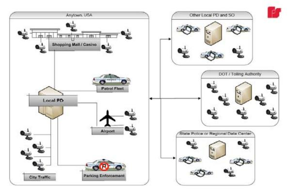
ALPR systems can generate vast amounts of data. The Federal Signal BOSS system is designed to enable law enforcement agencies to organize and archive data collected from multiple mobile and fixed site ALPR deployments.
