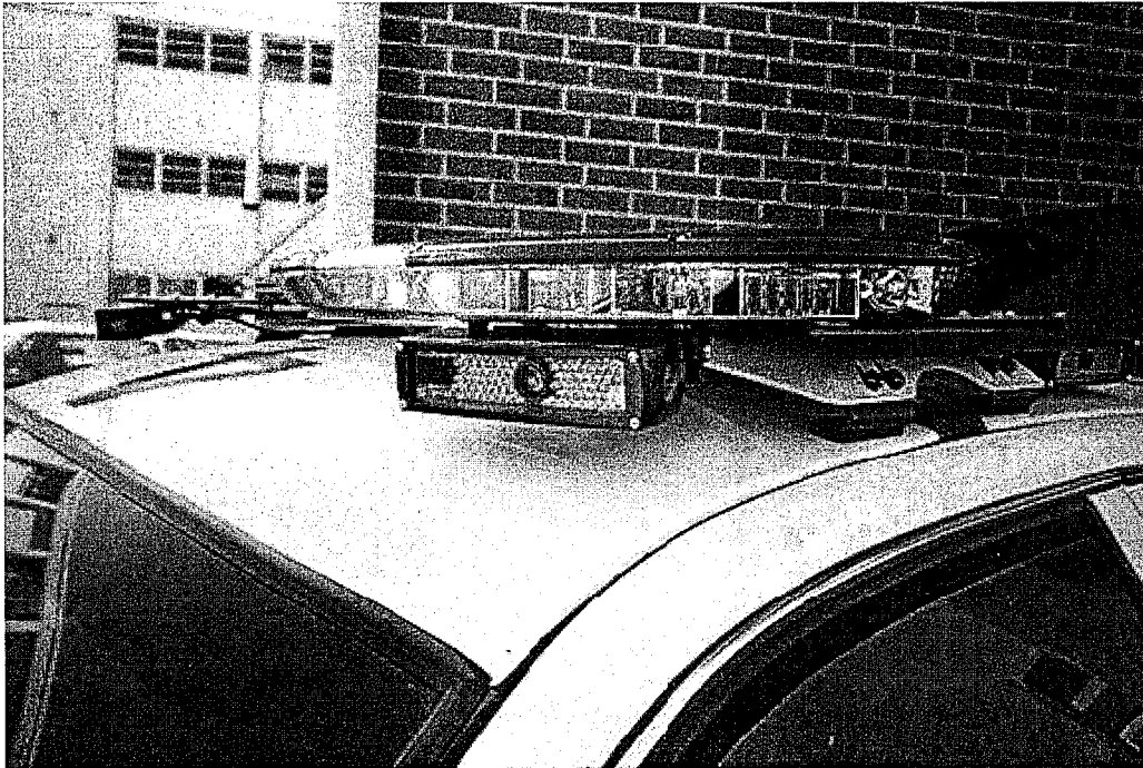
Figure 2-1: The low-profile Slate ALPR camera (up to four) unit mounts outside the vehicle under the lightbar
