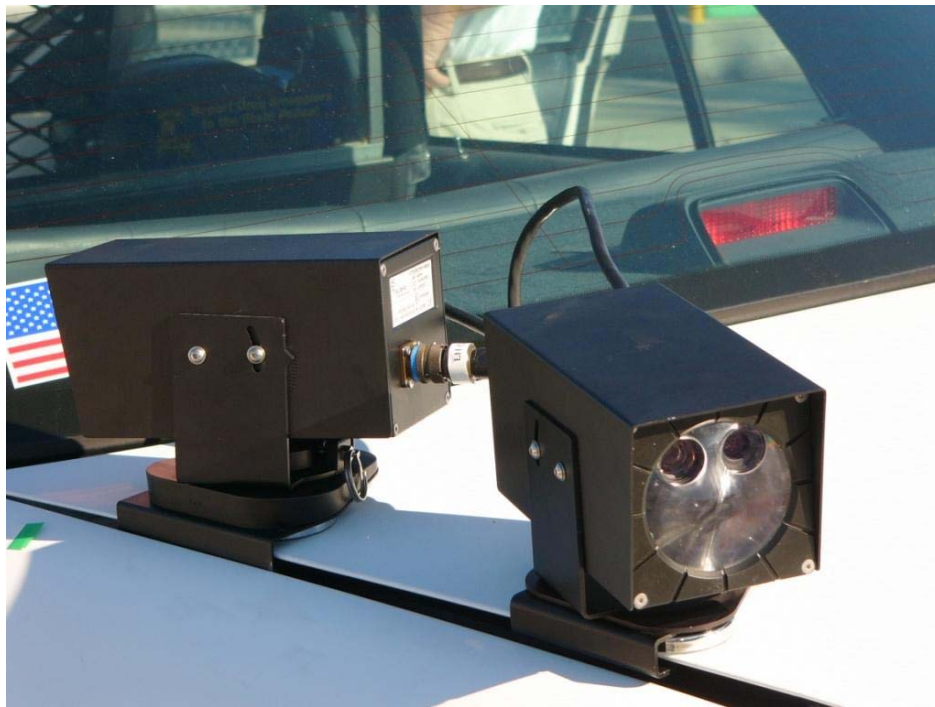
Figure 2: Example of trunk-mounted cameras.
