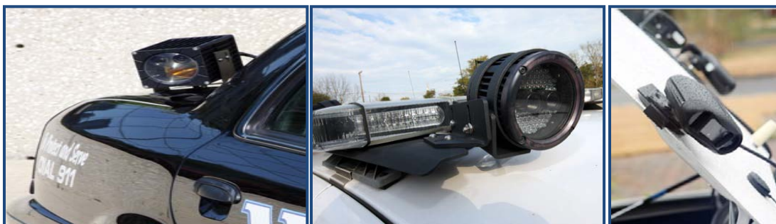
Figure 4: Examples of Trunk and Lightbar Mounted Mobile ALPR Cameras
