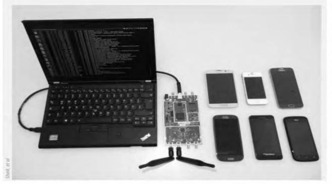
"The equipment can cause all LTE-compliant phones to leak their location to within a 32- to 64-foot radius ... operating a rogue base station... total cost" ... about \$1,400
