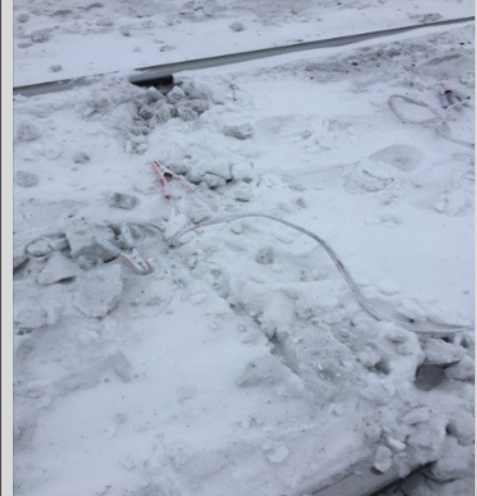
(U) Figure 2. Use of jumper cables to disrupt rail signals in North Dakota in January 2017. 77
