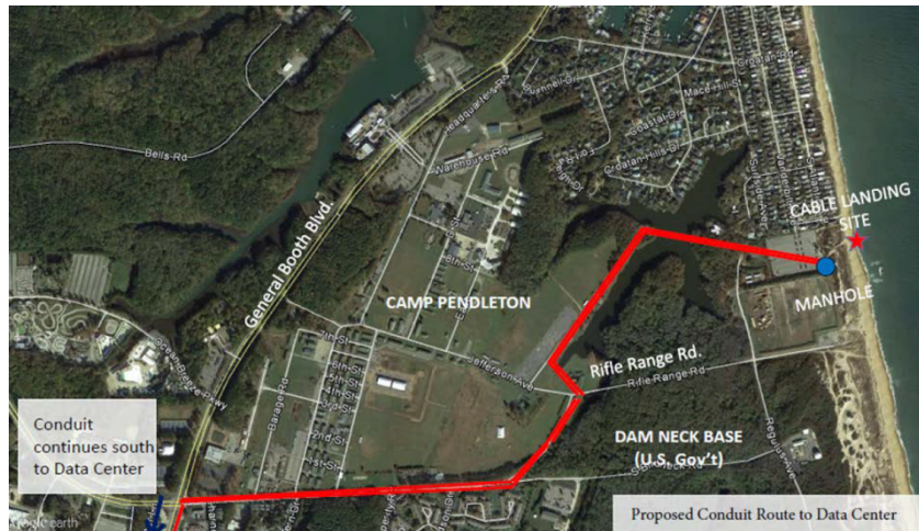
Figure 30 — Conduit path for MAREA cable 49
