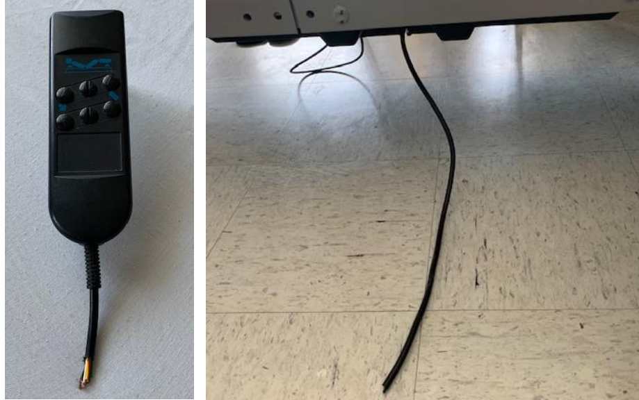
(Photographs 146-147: broken remote and wire, bed H-33, room 308)
